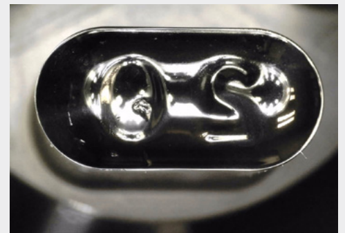
PUNCH TIP DAMAGE PHOTO TAKEN WITH IN 7950
