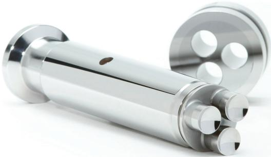
For full understanding, we needed to find the effects of different main and pre-compression forces on tablet quality and hardness. The analysis showed that compression forces over 19 kN, recreated the capping and sticking issues. Knowing the customer's growth plans, a multi-tip tooling design was recommended to increase production and reduce cost.
