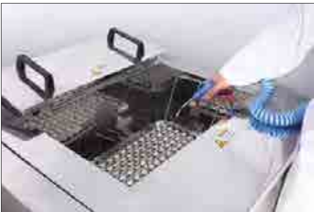
Drying wand blows hot air directly into punch heads and vented caps
