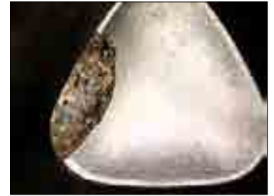
Punch Tip Damage Photo Taken with IN 7951
