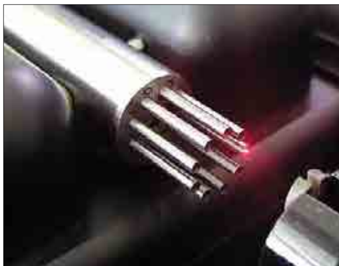
Laser Vision System (LVS) laser focused on a multi-tip punch
