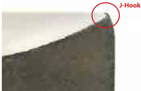
Punch with J-Hook wear
