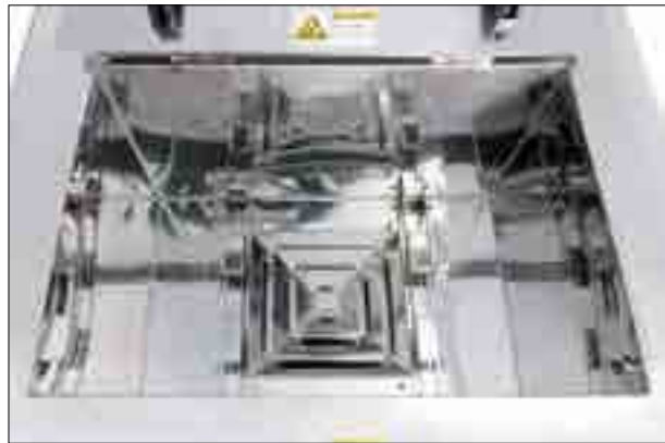
Drying unit blows air into punch cups
