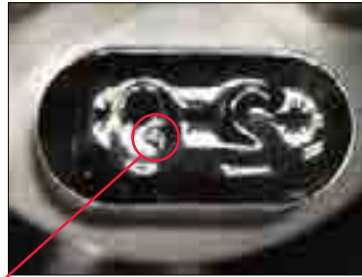
Punch Tip Damage Photo Taken with IN 7951
